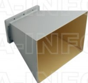
LB-650-10-A Standard Gain Horn Antenna 1.12-1.7GHz 10dB Gain Rectangular Waveguide Interface
